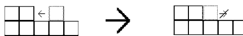
FIG. 4. Breaking of detailed balance by single-particle diffusion. A particle diffuses to the edge of an island where it sticks irreversibly. This process cannot be reversed so that detailed balance is broken.
